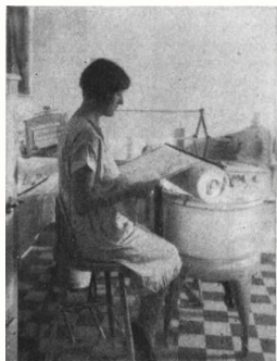
Wringer and ironer on this washer are interchangeable
